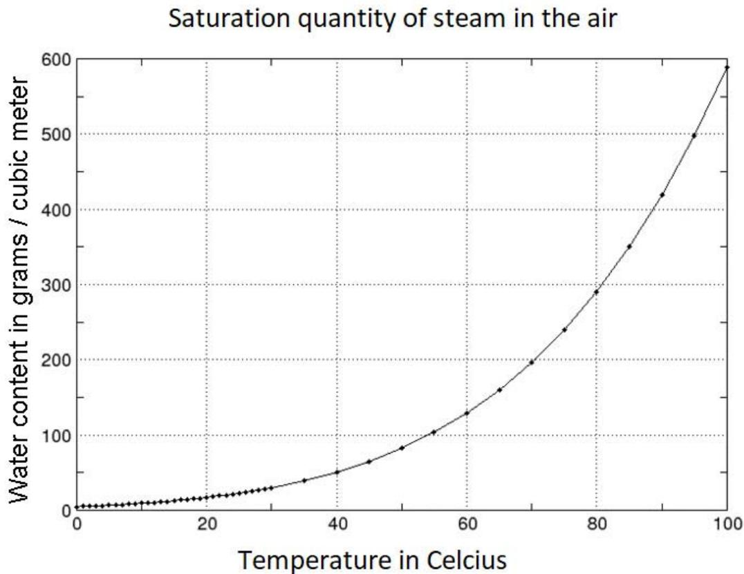
**Keep in mind:** The dew point has to be 15°C under the environmental temperature, otherwise the air will lose its ability to keep the water when being compressed. Water in the valve / actuator would then freeze and lead to leakage or malfunction.
