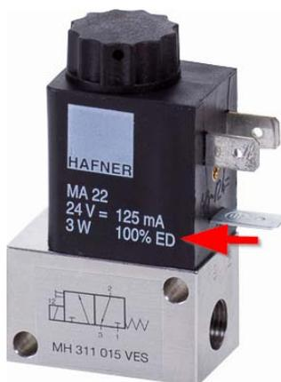
For solenoid valves the duty cycle specifies the maximum time of energizing the coil. The duty cycle is indicated as “ED” on the solenoids. Most of the Hafner solenoids are 100%ED what means that they can be energized continuously. For applications with 100%ED we recommend the usage of FKM plunger seals. NBR is hardening through and therefore not recommended. Hafner solenoid valves have FKM plunger seals as a standard.
