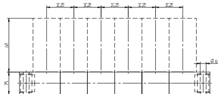
Parts of modular manifold RB 5 __ 121 G
