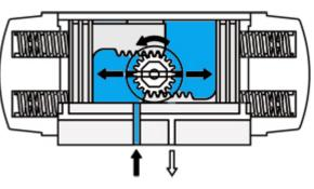
That is why in process automation, we aim towards an **air recirculation** into the spring chamber, also called a **"purge".**
