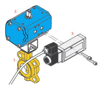
**1. Process valve** Part of the pipe-line system, e.g. ball valve or butterfly valve.
