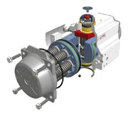
The 2 piston rods of the 2 pistons inside the actuator are shaped like racks. Compressed air is driving them. The racks drive a pinion which is linked via a shaft to the process valve and opens or closes it.
