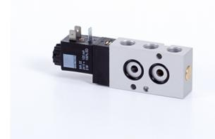
The picture displays a **MNH 510 701**, which is a **5/2-way** single solenoid NAMUR-valve. It is used to control a double-acting actuator.
