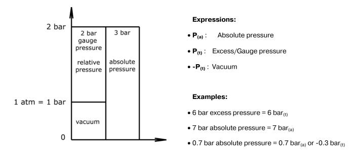
The expressions "excess pressure" and "vacuum" refer to a value larger or smaller than standard atmospheric pressure.
